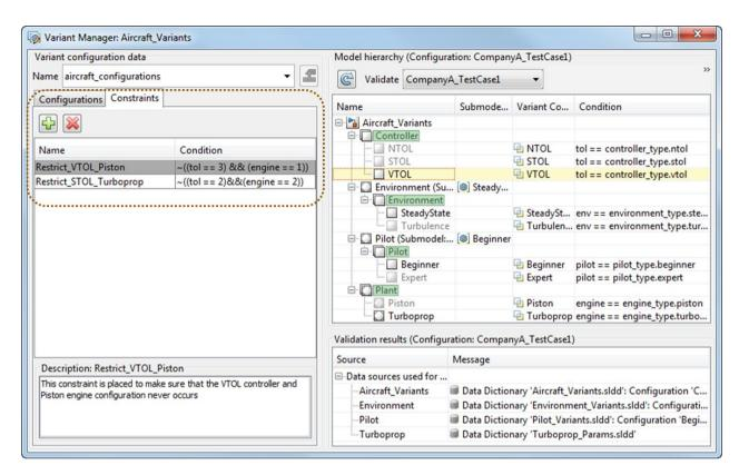
Figure 9: Define constraints using Simulink Variant Manager user interface
