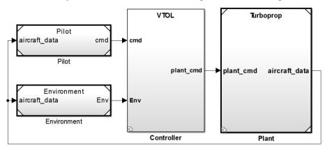
Figure 4: System level model Aircraft\_Variants showing the configuration requested by Company A
