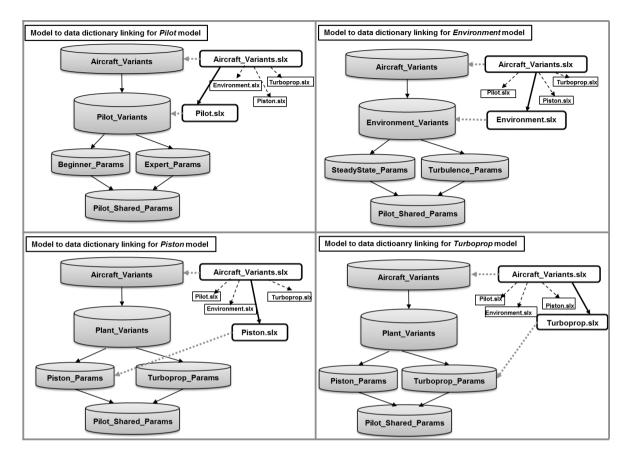
Figure 13: A data dictionary hierarchy does not necessarily correspond to model reference hierarchy
