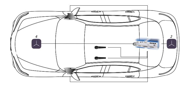
6 Accelerometers; 2 Loudspeakers; 2 Microphones
