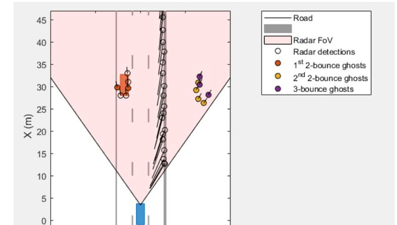
[Simulate Radar Ghosts due to Multipath Return](#)
