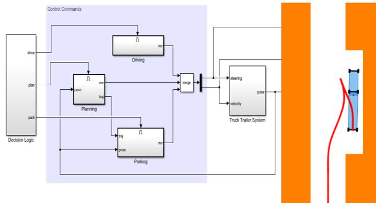
[Parallel Parking of Truck Trailer Using Multistage Nonlinear MPC](#)
