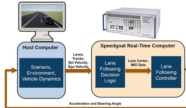
[Automate Real-Time Testing for Highway Lane Following Controller](#)
