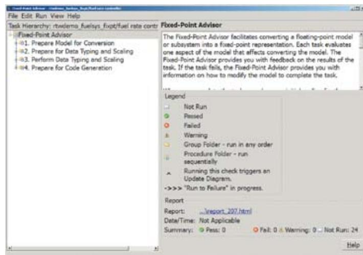
Figure 1. Model preparation using Fixed-Point Advisor.
