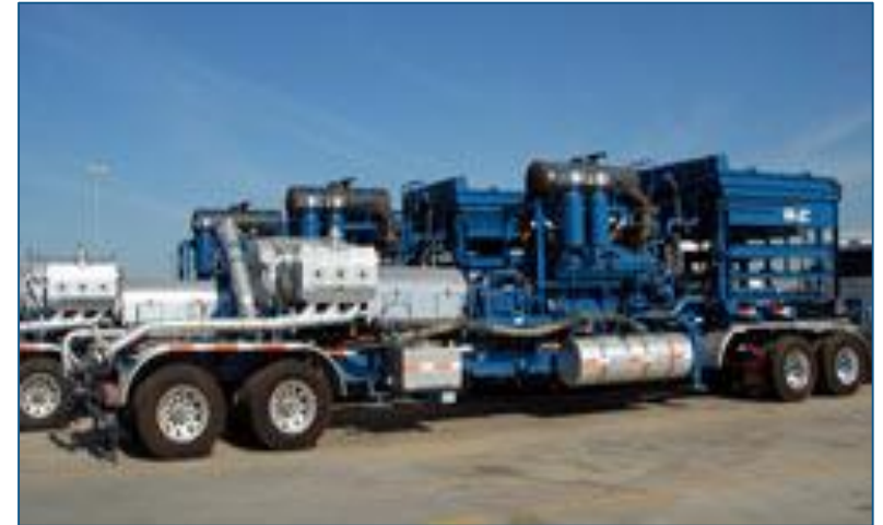
Truck with positive displacement pump.
