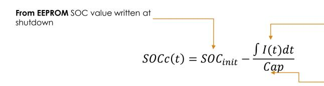
**High-Accuracy Current Sensor** with independent secondary current sensor and current rationality check in place to avoid large current accumulation error in single charge-discharge cycle
