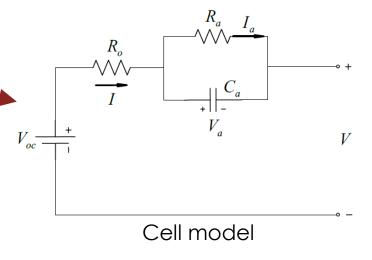
$$\dot{V}_a = -\frac{V_a}{R_a C_a} + \frac{I}{C_a}$$
